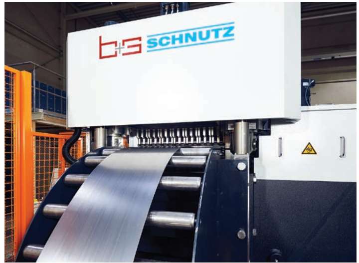
The new Schnutz machines at Adient each consist of a leveler with integrated feed unit, coil lift truck, decoiler, loop equipment and appropriate automation including safety devices.
